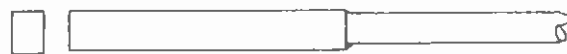
SNAPPER - wider than bottom of cutter, no higher than needed sharp edges
