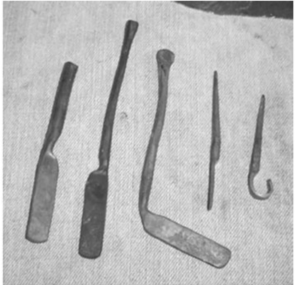
Use a half face blow to create a transition to about a 1" flat section.
