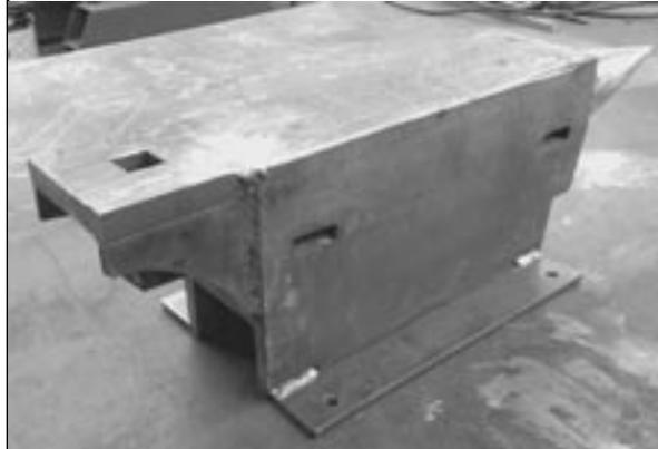
Finally Bob forged the horn from a piece of large stock and welded it on.
