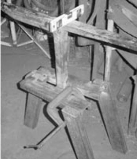
Then with two legs tacked in place and the third held in place with a "C" clamp I checked to make sure that the tool would be level when every thing was welded in this position.
