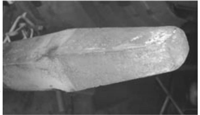
With all the pieces cut and clamped to the end of the stake, I tacked the corners and checked the alignment. When I was satisfied that it was a good fit on the end of the stake I welded the full length of each of the seams. Thus the socket was done. In the picture to the right you can see the progression of pieces going counter clockwise around the socket starting at the bottom piece.
