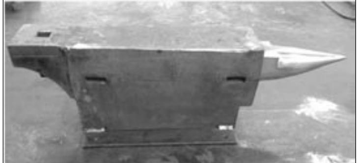
The heel is made from a treadle hammer anvil plate which already had the hardie hole cut in it to hold the treadle hammer dies.
