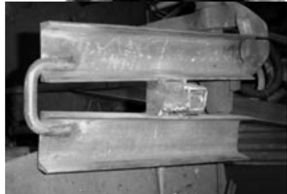
At this point I checked the alignment by putting the stake tool on my anvil up side down and dropping the platform into place. I took measurements from the platform to the anvil to make sure the socket was square with the platform.
