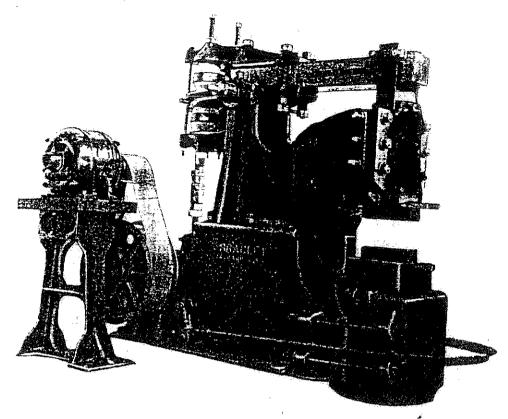
Bradley Upright Helve Hammers readily adapt themselves to an electric motor drive. The advantages of a motor driven hammer are many, but those which appeal more generally to the purchaser are that the hammer may be located in the most convenient place for use, irrespective of main line shaft, and also when not in use, no power is consumed.
