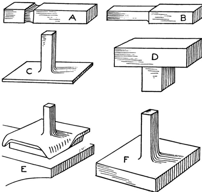
*Fig. 79. Method of Forging a Base*
