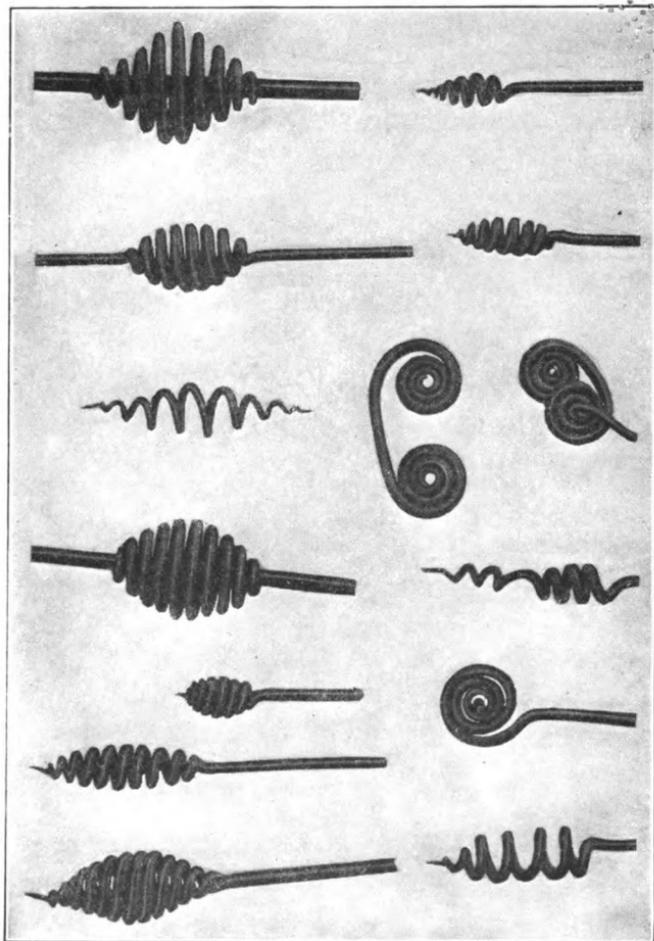
*Fig. 52. Spindle-Shaped Spirals*
