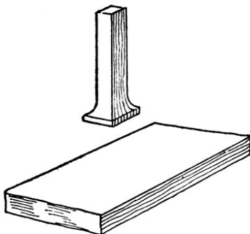
*Fig. 35. Stock for a Jump Weld*
