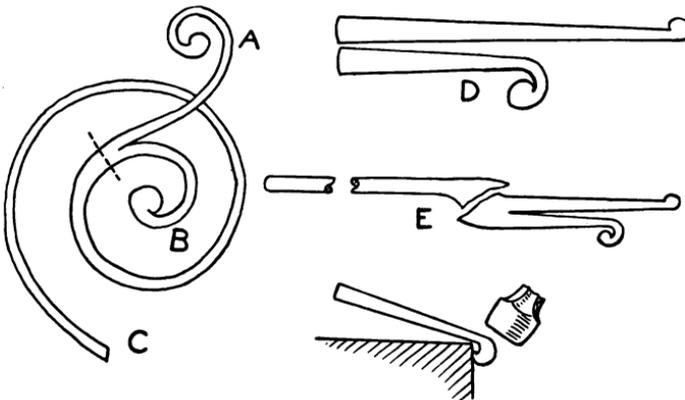
Fig. 76. Method of Welding Scrollwork
