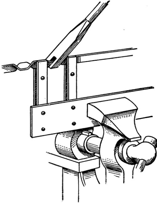
*Fig. 48. Twisting Flat Bars*
