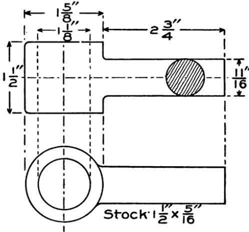
Fig. 41. Welded Eye from Flat Stock
