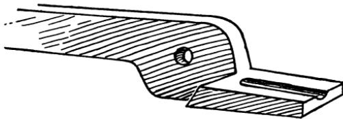
*Fig. 6. Jaw with Fuller Mark*
