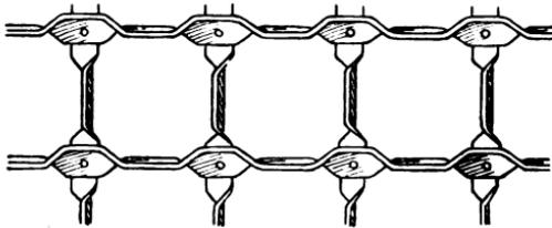
*Fig. 49. Mesh of Twisted Flat Bars*
