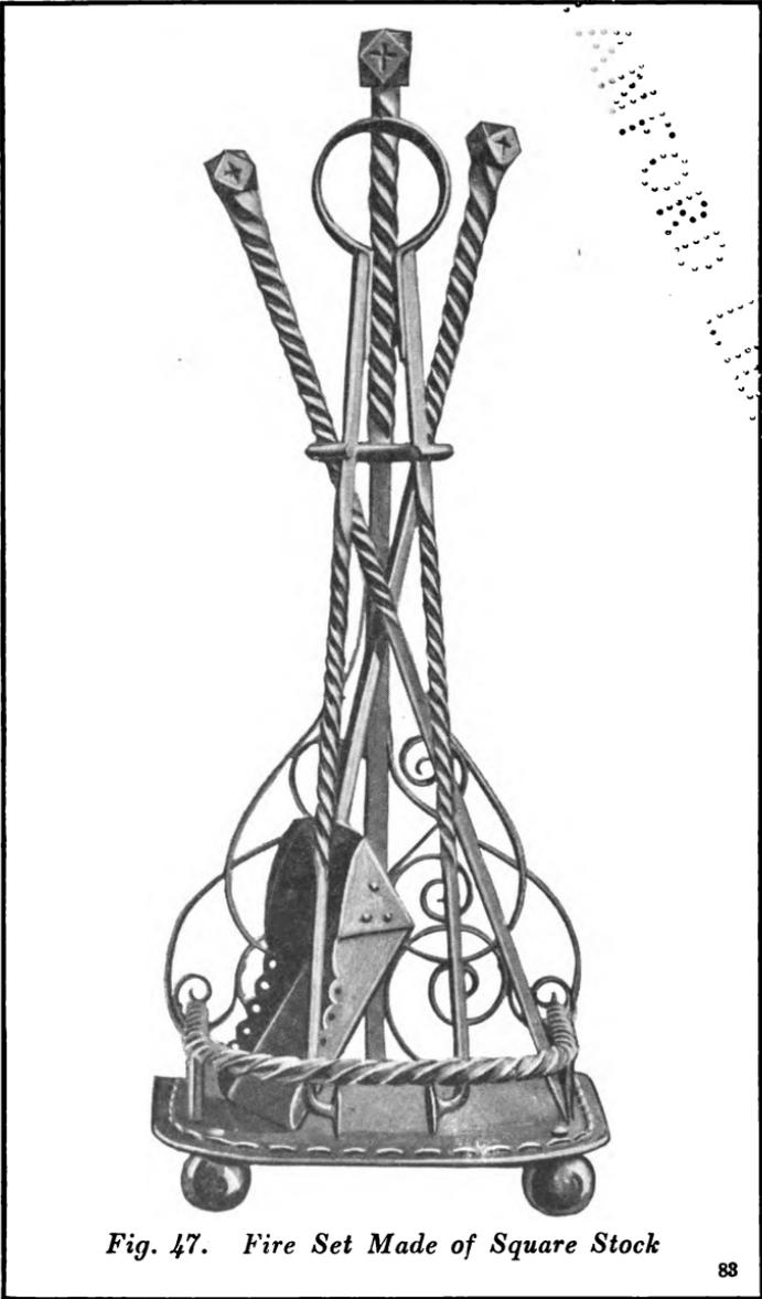
*Fig. 47. Fire Set Made of Square Stock*
