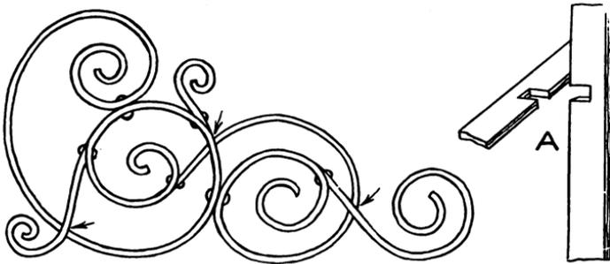
*Fig. 64. Riveted Scrollwork*
