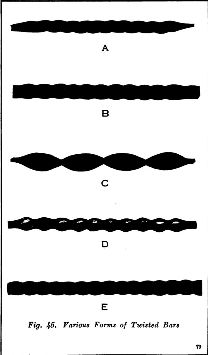
to a uniform heat and twisted. Twists of this kind, with possibly more bars, make very nice handles for pokers and shovels. At B a piece of  $\frac{1}{2}$ -in. square iron is twisted. At C a piece of
