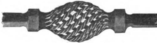
*Fig. 57. Bulb in Center of Bar*
