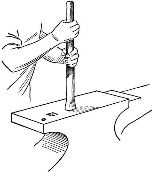
*Fig. 15. Upsetting by Ramming*
