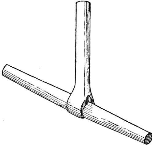
*Fig. 30. The Welded Joint*
