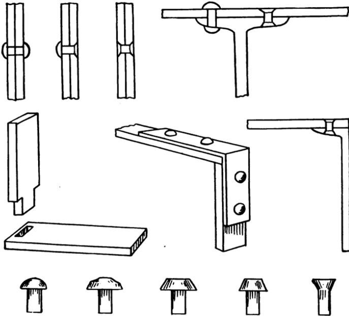
*Fig. 63. Methods of Riveting*
