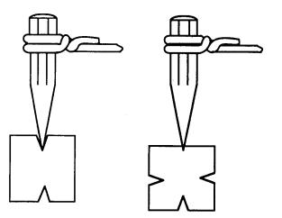
for the full length and turn over to the opposite side. Keep all cuts centered and keep the cutter vertical.
