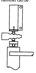
Grooving a flared fishtail with a hand held fuller is quickly done. Mark the desired grooves on the flare and fuller the grooves by walking a hand held fuller. The fuller may be narrow or wider, depending on the effect desired.
