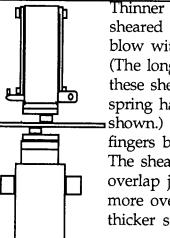
Thinner stock may be sheared with one hammer blow with spring shears. (The long spring handles of these shears, or most other spring handled tools, are not shown.) Don't get your fingers between the handles. The shear blades should overlap just slightly, with more overlap required for thicker stock.
