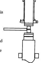
A swage may be made with a starter section and a finish size hole. This swage should be made from tool steel. Clamp a business card between the two swage halves and drill two holes (finished tenon size). Drill a larger size (about 1/8" larger) hole from the back on the starter side but don't drill through. Leave about 1/16" not drilled with the larger drill. Grind the sides of the drilled holes away on both holes. Grind about twice as much as you think is required.
