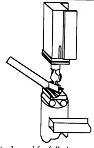
Get a smooth finish by using a flatter on flat or tapered stock. The hammer and anvil hard plates may be used as flatter on
