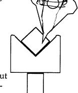
The tool will be kicked out to one side unless a vertical line can be drawn through the point and the
