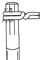
Slit part way from one side and then finish from the other side. Be sure slits are centered from side to side and ends line up with each other.
