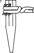
the hole and get stuck. Sometimes hammering on the side of the stock with a stuck punch in the hole will loosen it. Turn the stock on edge and hammer between the TH hard plates. Grind any mushroom ends off your punches before use.
