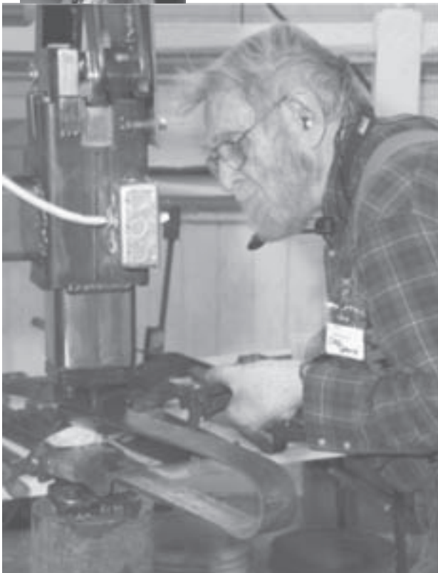
Left, Forging cut off hardie using his tire hammer.
