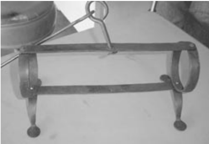
Pipe kiln, used to dry clay pipes
