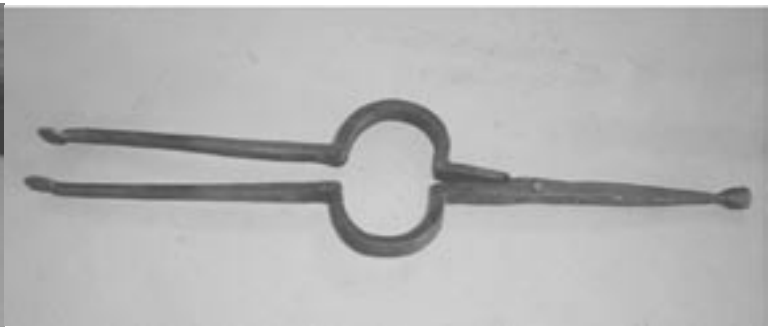
Pipe tongs with hidden box joint
