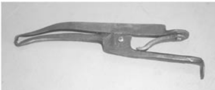
Striker tongs, hold char cloth while the top is used with flint to make the spark
