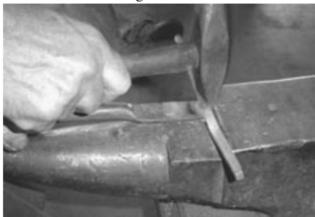
Above, Drawing out tabs on the female joint.
