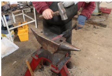
Ric Furrer forging a Knife from refined steel
