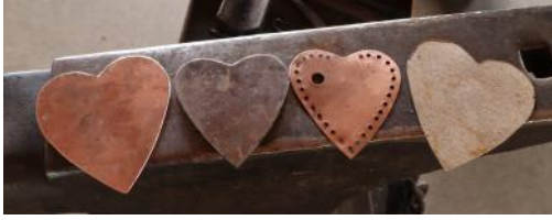
L to R Cut out copper blank, Shaping form, Hole pattern, Copper blank pattern
