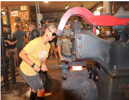
Kim Stahl welding a billet.
